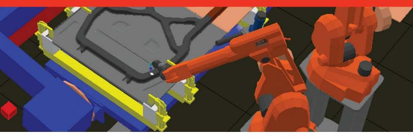
Nonstandard workcell components, such as custom fixtures and positioners can be quickly created in the built-in CAD package, or by importing CAD files via IGES, DXF, and direct translators.
