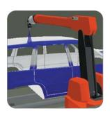
By evaluating the various robot movements and paint parameters in the digital environment, programmers can search for the optimal result without costly prototypes.
