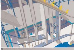
Close and prepare surfaces at WS 60 , parts (RbS\_1, R1\_R7\_front\_Spar\_1, R3\_R7\_frow\_Spar\_1)
